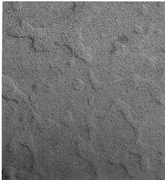
Figure 12 (a) Typical high-resolution image of the selective layer face (membrane MS14B). (b) Enlarged view of (a).
